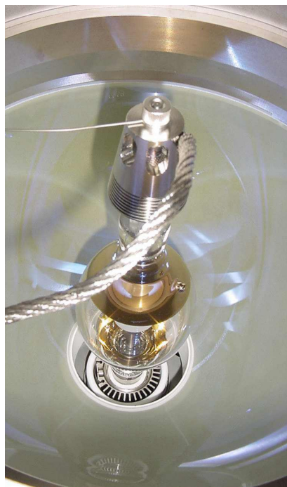
Figure 4.3 Lamp Mounted in Socket with thermocouple
