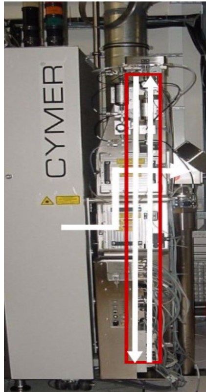
Figure 1.10 The Beam Shaping Module stretches the laser pulse in time by extending the path for parts of the beam.
