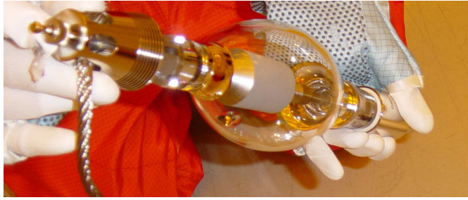
Figure 5.5 Reduce the risk of dropping the lamp by using two hands to hold it.
